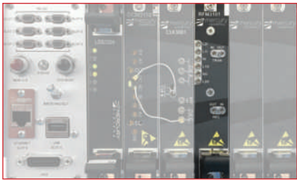
▲ Fig. 3 RFM3101 microwave transceiver integrated with an IF digital processing module, clock generation module and an Intel® Xeon®-based processing module, all supplied by Mercury Systems.
