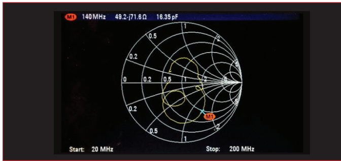
▲ Fig. 19 Measured S_{11} of an antenna for a VHF/UHF radio, from 20 to 200 MHz.
