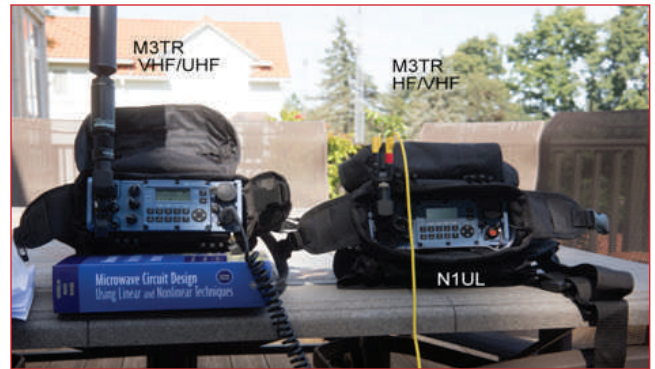
▲ Fig. 20 VHF/UHF (left) and HF/VHF (right) manpacks. The UHF/VHF manpack shown uses a thick vertical pole antenna, and the HF manpack uses a 5 m dipole (the yellow wire).
