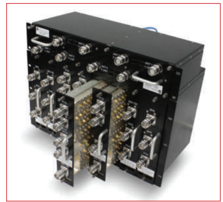
▲ Fig. 3 Neutral host small cell and D-RAN systems support several operators and must handle multiple carriers operating on different frequency bands.
