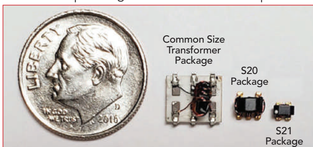
▲ Fig. 1 Common surface-mount transformer with soldered leads compared to S20 and S21 packages with welded leads. 5
