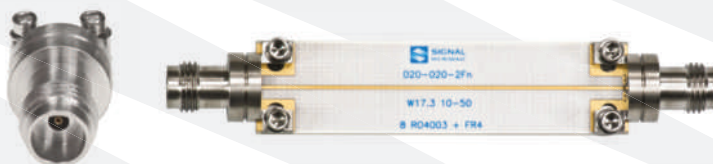
2" GCPW test board with typical data through 110GHz
